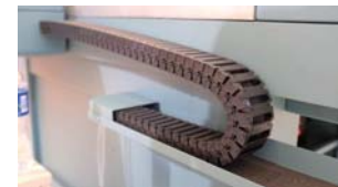
PU pad laid under the cable chain to reduce noise
