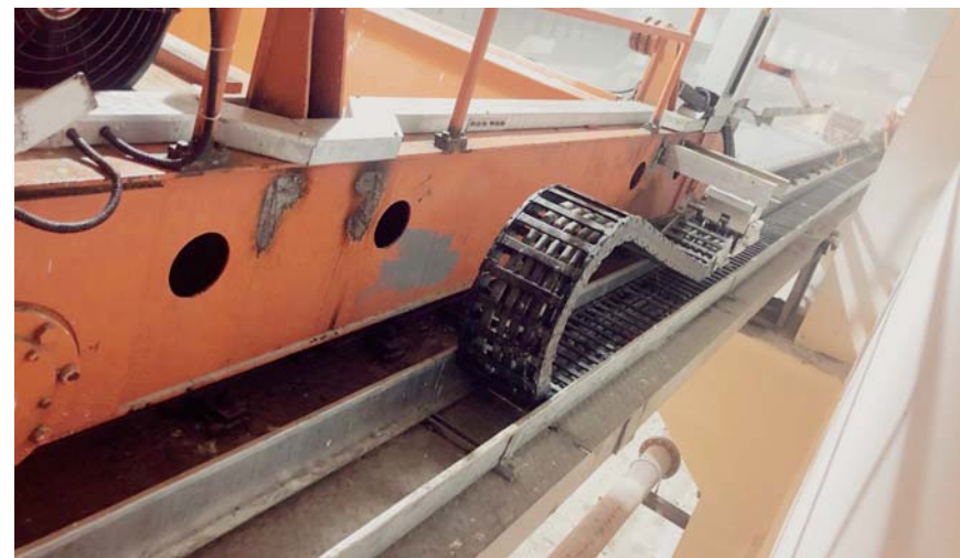
Long travel of 138m with systems GeMotion, GuidEasy guide trough and floating moving arm in condition of high temperature and humidity
